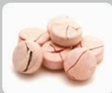
Example of Bad Tablet Coating
